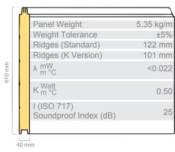
Panel weight is for indication purposes only. Due to the typical tolerances getted during the several steps of the panels components manufacturing process, variations in the final weight of the panel can be found. For this reason and in accordance with the industrial "Best Practices", Teosedo recommends to weigh the panels before using them for each door assembly, in order to choose the most suitable springs.
