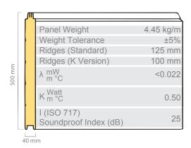
Panel weight is for indication purposes only. Due to the typical tolerances getted during the several steps of the panels components manufacturing process, variations in the final weight of the panel can be found. For this reason and in accordance with the industrial "Best Practices", Tecsedo recommends to weigh the panels before using them for each door assembly, in order to choose the most suitable springs.
