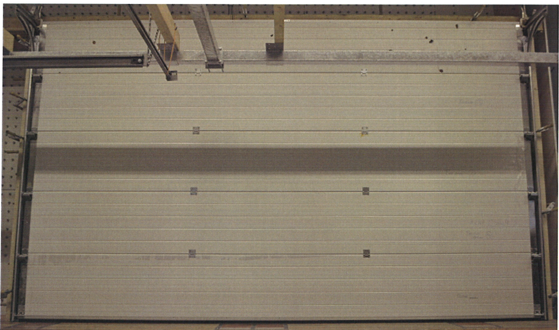
Figure 1. Door type DOCO SFR Tecsedo, mounted in the test rig, as seen from inside.
